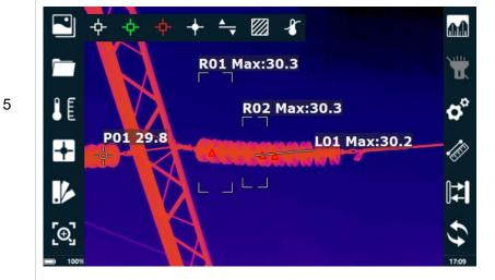
click to enable temperature difference analysis, to display the temperature difference between two regions.
