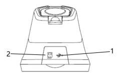
Figure 3.3 Illustration of Connector and Memory Card
