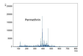
*Figure 3.* TD-ESI mass spectrum obtained by Portability from examined tomato. Permethrin m/z = 392
