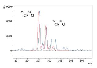
**Figure 6.** TD-ESI mass spectrum obtained by Portability from examined lemon. The zoomed spectrum shows chlorine isotopic distribution in ionized imazalil. Pesticide. Match with theoretical isotopic spectrum: Blue = experimental spectrum; Red = simulated spectrum
