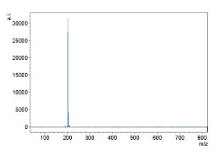
**Figure 5.** TD-ESI mass spectrum measured in Selected Ion Monitoring mode obtained by Portability directly from an orange surface. The only peak corresponds to pesticide thiobendazol at m/z = 202
