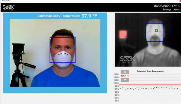
4. Blue box means the camera has detected a face and is measuring skin temperature.
