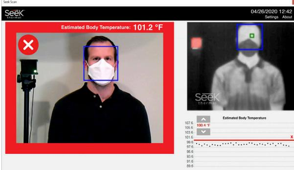
6. Red box means estimated body temperature is above the alarm temperature.
