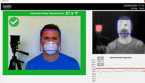
5. Green box means estimated body temperature is below the alarm temperature.
